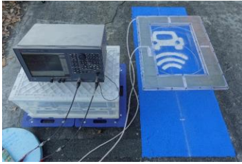
Fig. 16. Status of power transmission evaluation with VNA.
