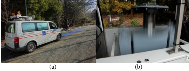
Fig. 21. Status of FWD test. a) FWD test car, b) Falling weight.
